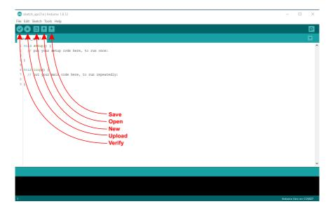
The function written in the "void setup ()" section in the program will only work once when the board is powered up. Input / output pins, serial port configuration etc. settings are adjusted in this section. The "void loop ()" section contains functions that will run continuously until the board is de-energized after running the commands in the "void setup ()" function.
