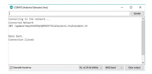
After setting the serial port speed to 9600, display the results coming from the Arduino. After the message sent text appears in the serial port, view the data via thingspeak.
