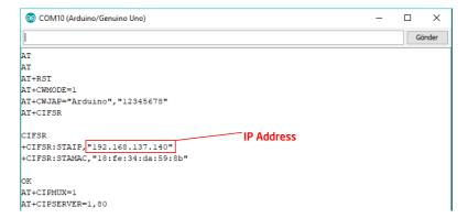
Open the serial port via Arduino IDE and set the data rate to 115200. Communication with the ESP8266 module can be seen here. When the above settings are made, connect to the IP address of the serial port with a web browser.
